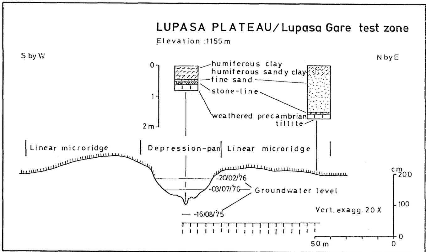
Figure 5 : Cross-section in a set of two linear micro-ridges and a depression-pan in the Lupasa Gare test zone on the Lupasa plateau (for situation, see Fig. 2).
